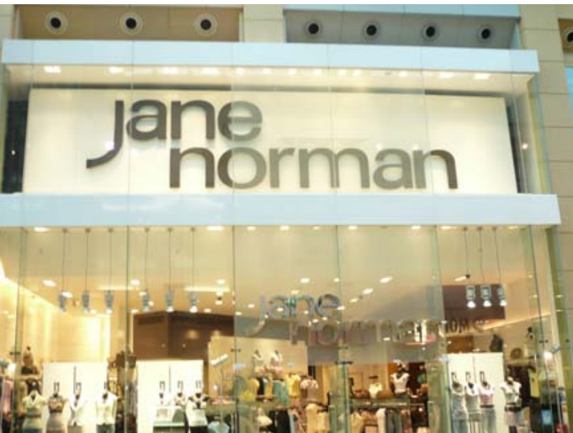
3. pushed through letters, internally illuminated
